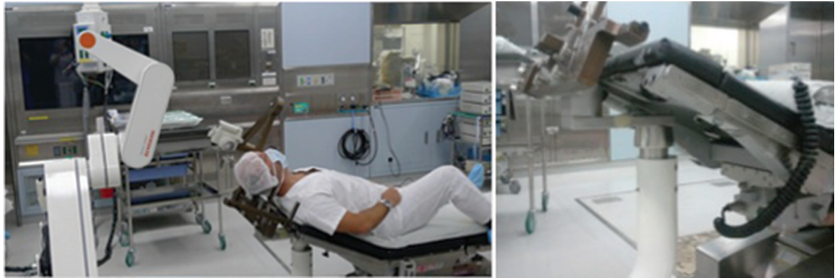
Fig. 3 The base of the patient's head position was tilted by 25 degrees to obtain an easy configuration by raising the back of the operating table.
