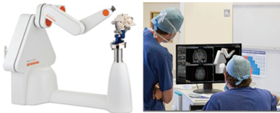
Fig. 1 The left photograph shows the neuromate robot system, including the five degree-of-freedom robotic arm assembly and personal computer-based kinematic positioning software system. The right photograph shows clinical preoperative planning image that was produced by the planning software (VoXim™, IVS Technology GmbH) at North Bristol National Health Service Trust Southmead Hospital in England.
