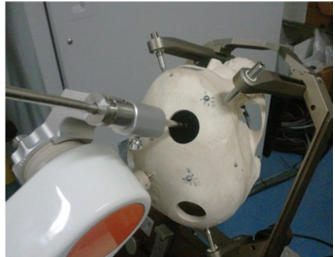
Fig. 5 The phantom was fitted with implantable markers. The markers were used to accurately measure the location of the probe tips placed according to each of the frame-based methods.
