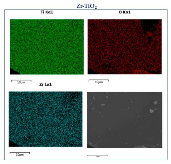
**Figure 4.** EDX maps over the Zr-doped sample.
