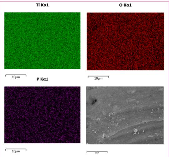
Figure 5. EDX maps over the P-doped sample.
