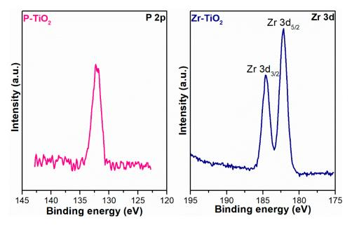
Figure 9. X-ray photoelectron spectra of P 2p and Zr 3d of P-TiO<sub>2</sub> and Zr-TiO<sub>2</sub>, respectively.
