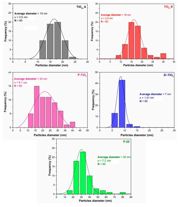
**Figure 3.** Particle size distribution of the samples studied.
