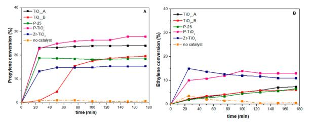
Figure 10. Trends of the propylene (A) and ethylene (B) conversions (%) over the time-on-stream.
