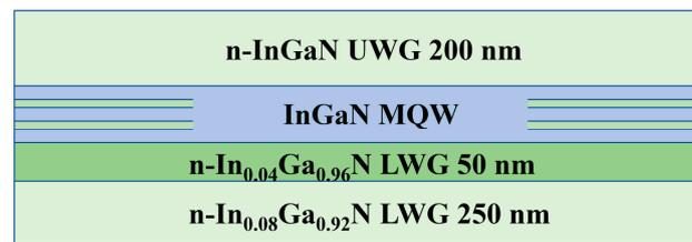
**Figure 6.** Schematical diagram for studied MQW and waveguide regions of a new LD structure with composite lower waveguide structure.
