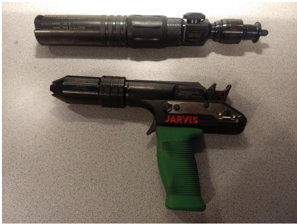
Figure 2. Examples of inline (top) and pistol (bottom) penetrating captive bolt devices. Inline device: Jarvis Model PAS Type C—0.25R Caliber, Super Heavy Duty (Order #: 4144059, Jarvis Corp., Middletown, CT). Pistol device: Jarvis Model PAS Type P—0.25R Caliber Captive Bolt Pistol (Order #: 4144035) with the Long Stunning Rod Nosepiece Assembly (Order #: 3116605).
