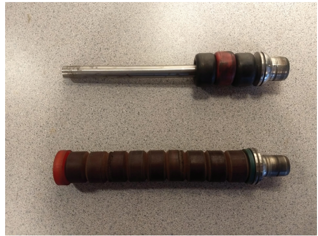
Figure 3. Examples of buffer system for free-flight (top) and self-retracting (bottom) penetrating captive bolt devices. Free-flight device: Jarvis Model PAS Type C—0.25R Caliber, Super Heavy Duty (Order #: 4144059, Jarvis Corp., Middletown, CT). Self-retracting device: Jarvis Model PAS—Type P 0.25R Caliber Captive Bolt Pistol (Order #: 4144035, Jarvis Corp.) with the Long Stunning Rod Nosepiece Assembly (Order #: 3116605, Jarvis Corp.).
