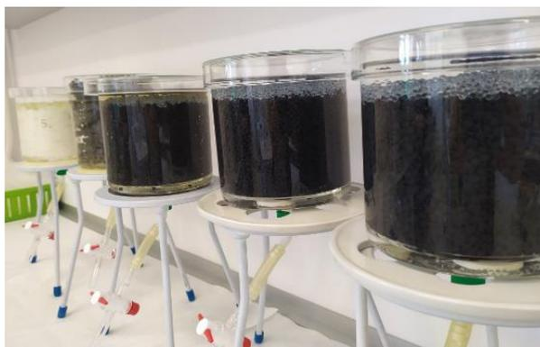
**Figure 1.** Testing for the release of ions and heavy metals from porous materials during leaching.
