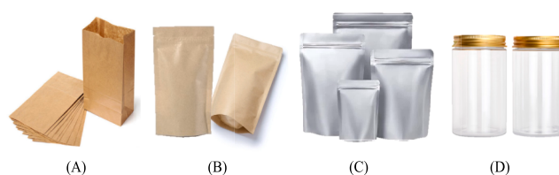
Fig. 1. Types of packaging used in the experiment: A) Kraft paper bag; B) bag of paper combined with polyethylene (PE); C) bag of aluminum combined with PE; D) jar of polyethylene terephthalate (PET).
