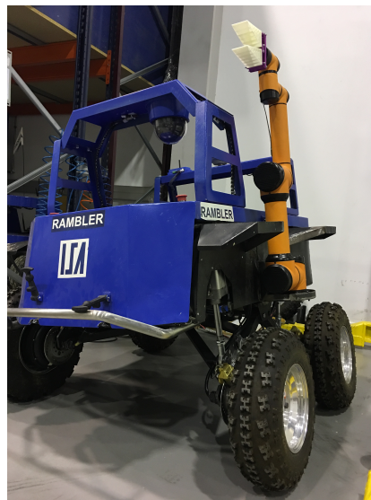
Figure 1. The all-terrain mobile robot for rescue applications, from the University of Málaga, showing the attached arm with a flexible adaptive gripper.
