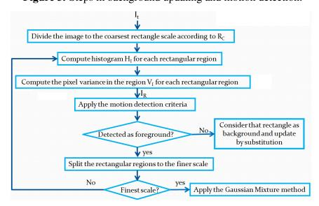
**Figure 3.** Steps in background updating and motion detection.
