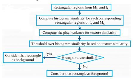
**Figure 4.** Motion detection criterion.
