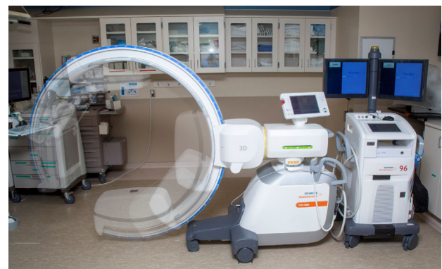
Figure 4 Rotation of the CIOS which ensures clearance of the anesthesia circuit, access, lines and other equipment. The proceduralist has unobstructed access to the patient's head.
