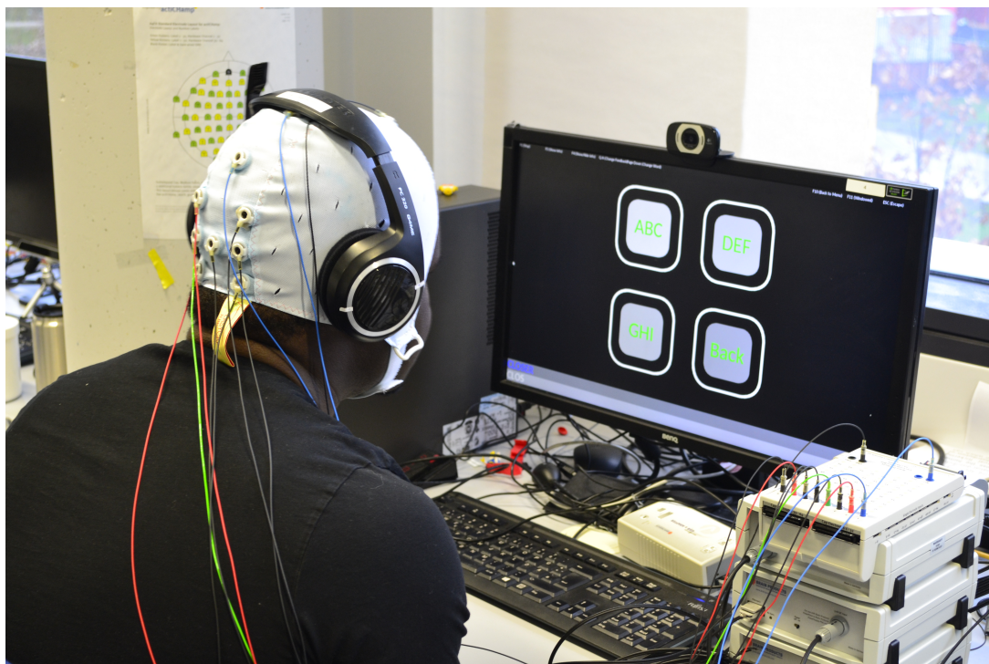
Figure 1. The setup of the experiment with the used 4-target interface. The amplifier, BrainAmp, is located to the right of the monitor.
