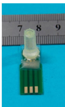
Figure 3. The photo of packaged dissolved oxygen (DO) microsensor.
