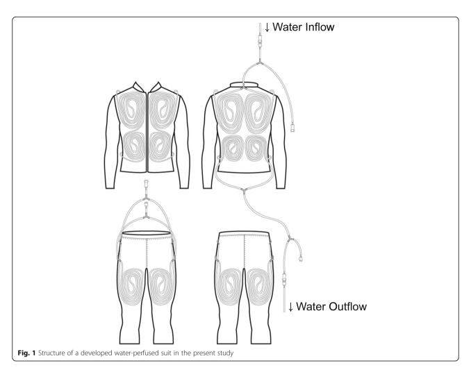
arms, legs, and feet) were not heated in order to optimize the water circulation rate. The suit was connected to a water bath circulator to heat the skin (RW-0525G, JEIO TECH, Korea, a resolution of 0.1 °C), with an average water flow rate of  $37.31 \pm 0.86 \, \mathrm{L} \, \mathrm{h}^{-1}$ .
