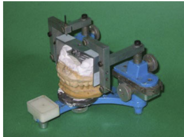
Figure 2 Mandibular position analyzer. The apparatus added to an articulator for the three-dimensional analysis of the mandibular position consists of right and left recording arms with pins into the condylar post holes. The recording frame is attached to the upper cast. The mandibular positions are recorded on the frame by the needles on both sides.
