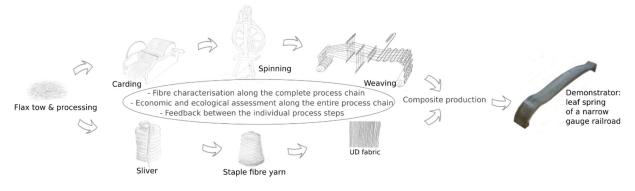
Figure 1. Process chain—from raw fibre to composite.
