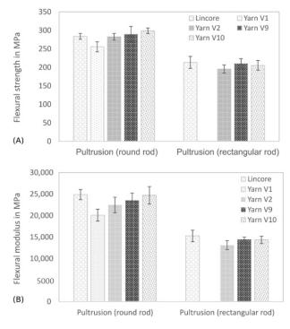
**Figure 7.** Flexural strength (**A**) and flexural modulus (**B**) of pultruded round and rectangular rods (fibre volume fraction of round rods ~40% and of rectangular rods ~30%). Results are shown as mean values with standard deviation as error bars.
