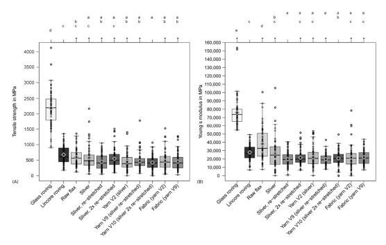
**Figure 6.** Properties of raw flax and single fibre bundles prepared from slivers, yarns and fabrics. (**A**) Tensile strength and (**B**) Young's modulus shown as box-whisker plots with rhombuses as mean values. Different letters indicate significant differences between the results. Results that are not normally distributed are marked with \*.
