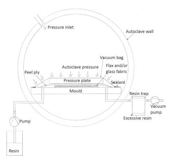
Figure 2. Schematic representation of the resin injection process in the autoclave (autoclave injection).
