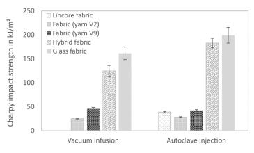
**Figure 14.** Unnotched Charpy impact strength of composites produced by vacuum infusion and autoclave injection. Results are shown as mean values with standard deviation as error bars.
