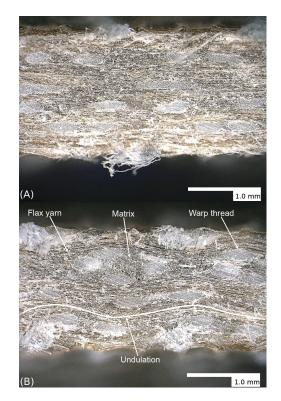
**Figure 10.** Micrographs (Keyence digital microscope VHX 6000, Osaka, Japan) of **(A)** composite laminates manufactured from the Lincore fabric and **(B)** a flax fabric (yarn V9) in a longitudinal direction.
