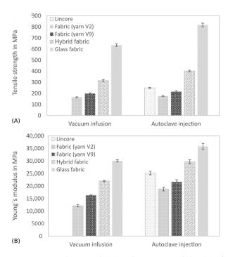
**Figure 9.** Tensile strength (**A**) and Young's modulus (**B**) of composites produced by vacuum infusion and autoclave injection. The results are shown as mean values with the standard deviation as error bars.
