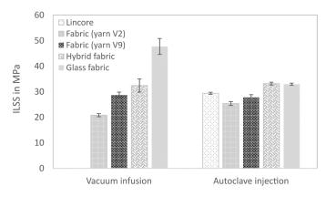
**Figure 13.** Interlaminar shear strength (ILSS) of composites produced by vacuum infusion and autoclave injection. Results are shown as mean values with standard deviation as error bars.
