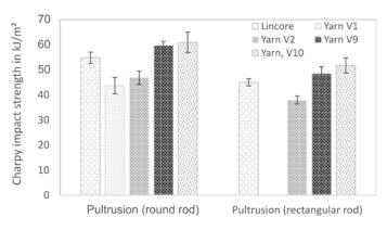
**Figure 8.** Unnotched Charpy impact strength of pultruded round and rectangular rods (fibre volume fraction of round rods ~40% and of rectangular rods ~30%). Results are shown as mean values with standard deviation as error bars.
