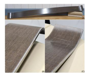
**Figure 15.** Prototype of a flax fibre-reinforced leaf spring of a bogie of a narrow-gauge railway produced by RTM, (**A**) overview, (**B**,**C**) detailed images (width of the leaf spring: 90 mm, length: 1170 mm).
