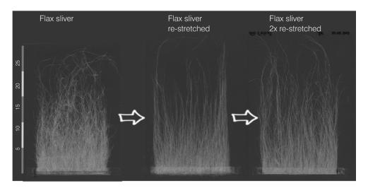
Figure 5. Length distribution depending on re-stretching of the sliver.
