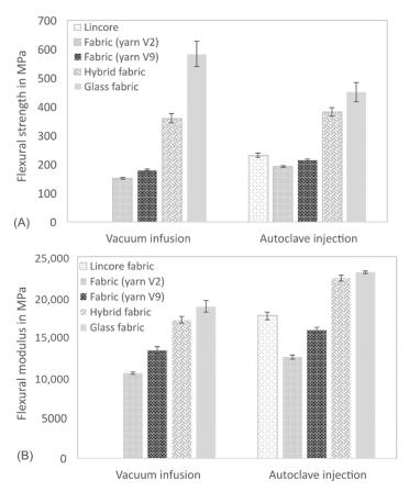
**Figure 11.** Flexural strength (**A**) and flexural modulus (**B**) of composites produced by vacuum infusion and autoclave injection. Results are shown as mean values with standard deviation as error bars.
