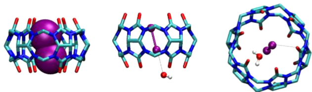
Figure 97. Stick-style views of the single-crystal X-ray structure of the cucurbit[6]uril–I 2 complex. Encapsulated diiodine, in space-filling style (left), is halogen-bonded with a water molecule (middle) and is bound to the carbonyl oxygen at the upper portal (right).
