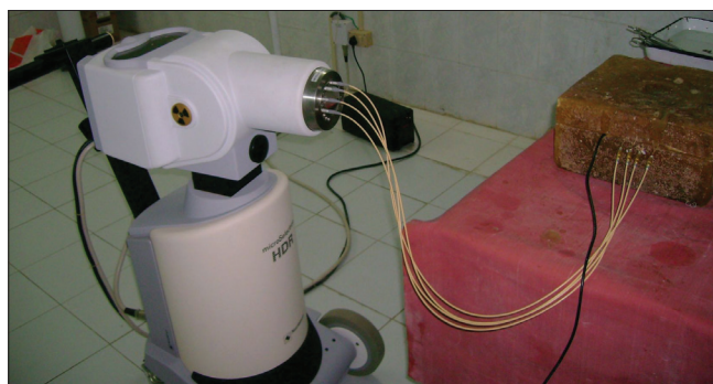
Figure 2: Pictorial view of the micro HDR connected with wax phantom and 0.015cc PTW ion chamber
