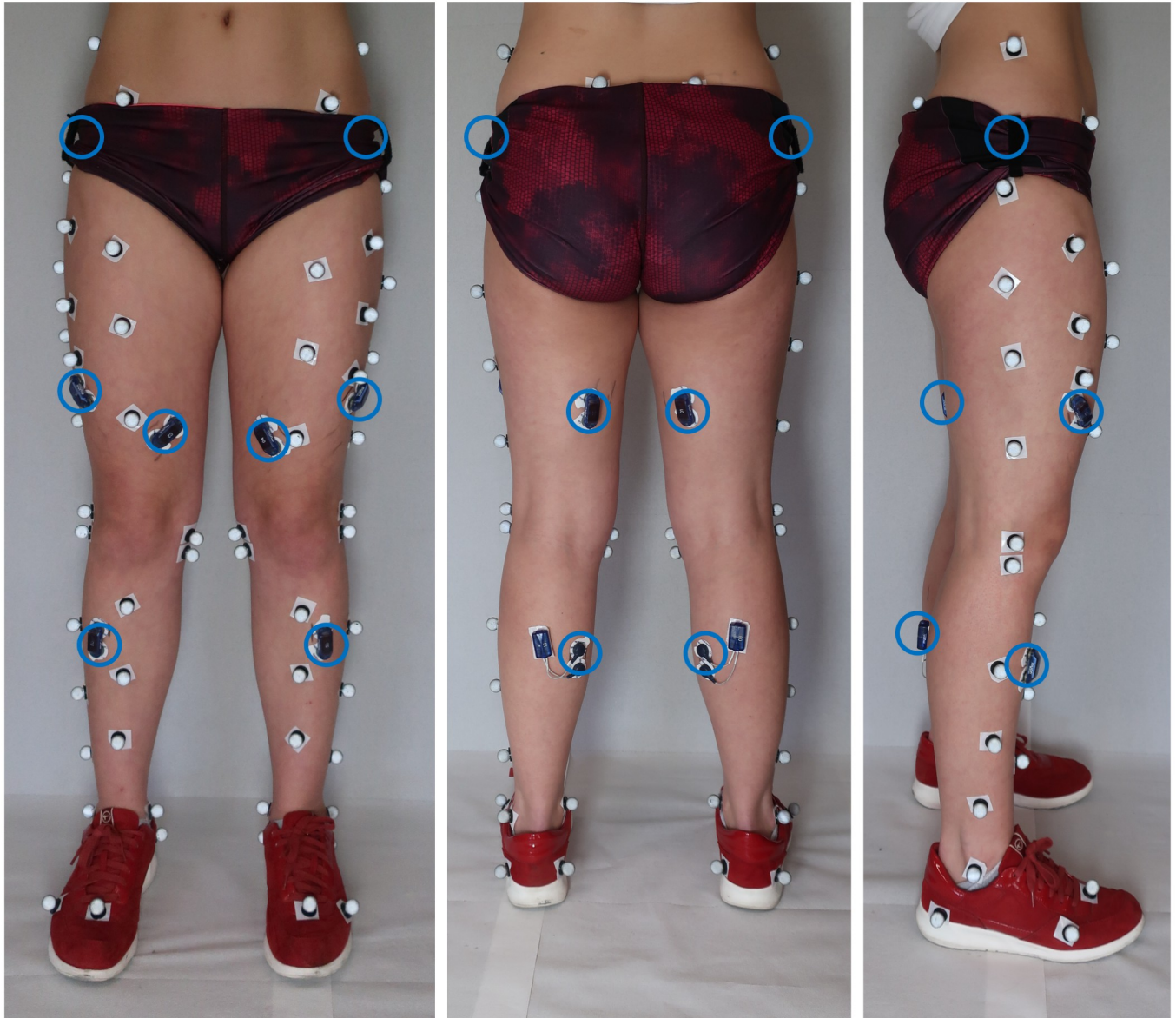
Fig 4. Marker and electromyography electrodes placement during the biomechanical assessment. Surface electromyography electrodes (blue circles; electrodes on gluteus medius under the pants) and marker placement (bright dots) for 3D motion analysis in front (left), back (middle) and side (right) view.
