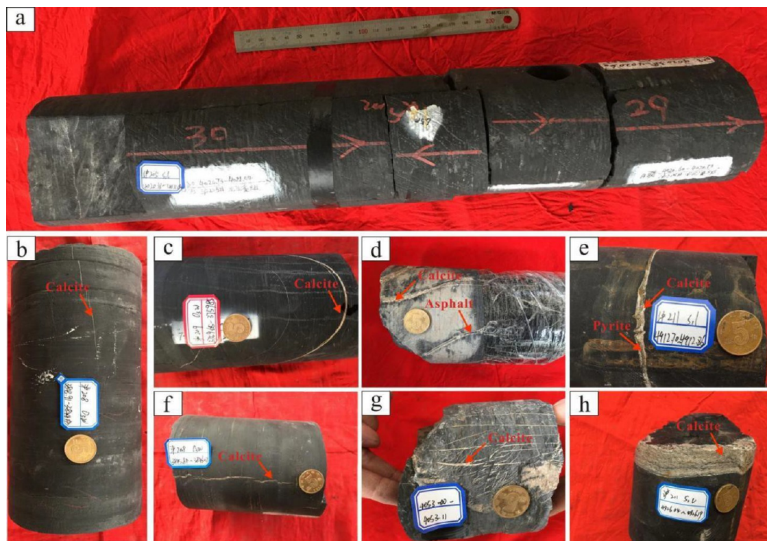
Figure 2. Core fracture characteristics of Wufeng–Longmaxi Formation in L203 Well area. (a) Upright shear fracture, unfilled, Well L205, 4020.38~4021.04 m. (b) Upright shear fracture, filled with calcite, Well L208, 3843.91~3844.14 m. (c) High-angle shear fracture, calcite fully filled, Well L209, 3759.65~3759.85 m. (d) Tension fractures, fully filled with calcite and asphalt, Well L206, 4053.43~4053.68 m. (e) Horizontal fractures, fully filled with calcite and asphalt, Well L211, 4912.70~4912.86 m. (f) Tension fracture, filled with calcite, Well L208, 3845.84~3846.026 m. (g) Abnormally high-pressure fracture, filled with calcite, Well L206, 4053.00~4053.11 m. (h) Dissolution fracture, filled with calcite, Well L211, 4926.04~4926.19 m.
