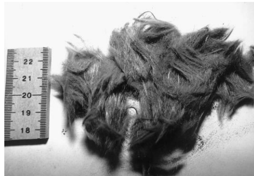
Figure 11. Glass fiber recovered from the fluidized bed process, [51].
