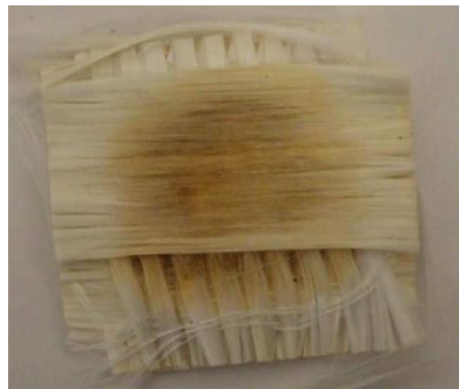
Figure 13. Sample (50 × 50 mm) after hydrolysis at a temperature around 300 °C [26].
