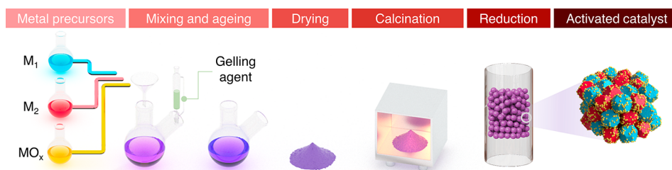
Figure 2. Sol–gel synthesis procedure developed for M_{1\alpha}M_{2\beta}@MO_x-\gamma catalysts. Synthesis steps are detailed in the Experimental Section.
