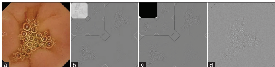
Figure 4: A decomposed image with three-level “sym10” wavelet transform (WT). (a): Original image, (b): Three levels of decomposition in the two-dimensional discrete WT, (c): Transform modified by zeroing the LL subband, (d): Reconstructed edge image
