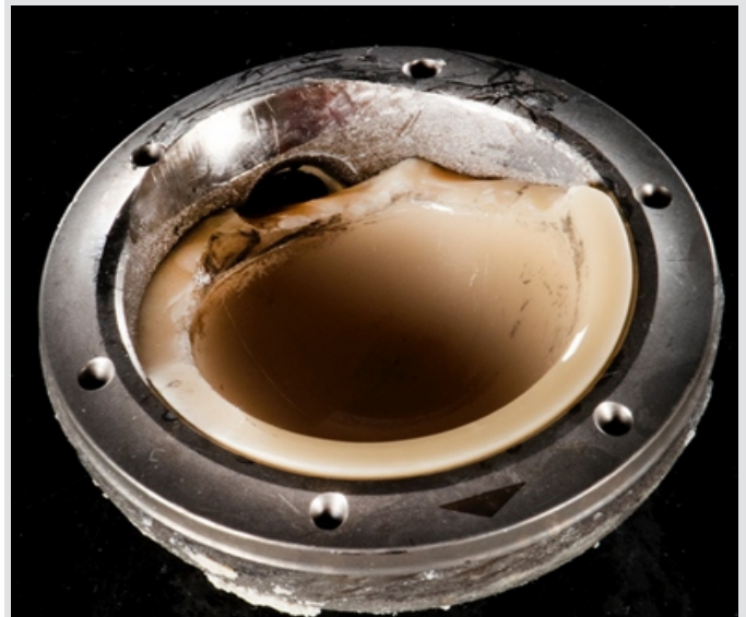
Figure 2: Clinical photograph showing wear of superolateral aspect of ceramic acetabular component.
