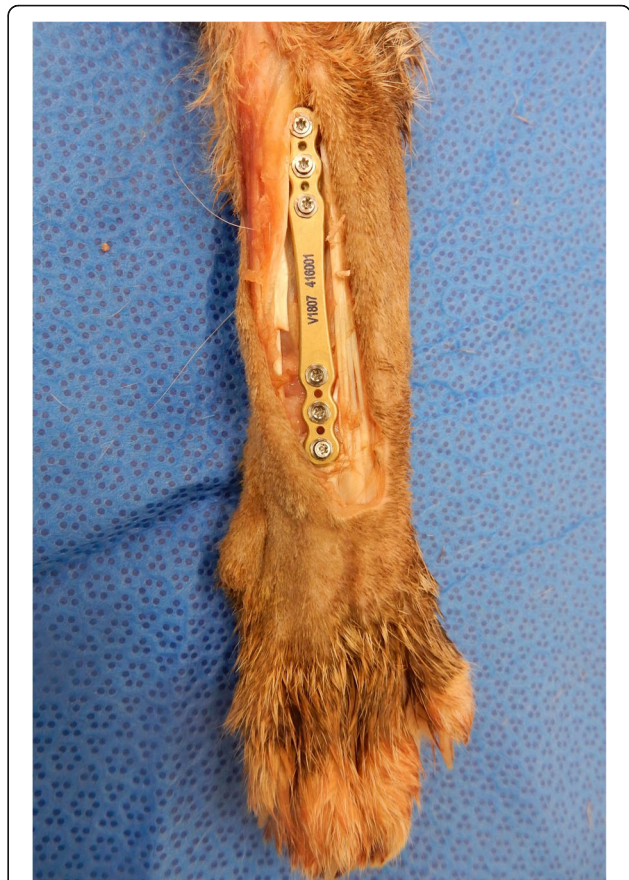
Fig. 3 Image for demonstration of a test specimen without placement in the testing jig. Dorsal approach to the distal radius and carpus has been made, and a six hole, 1.7 mm conical coupling locking plate is secured to the bone with the three most proximal screws engaging the radius, the fourth screw engaging the radial carpal bone and the two most distal screws engaging metacarpal III
