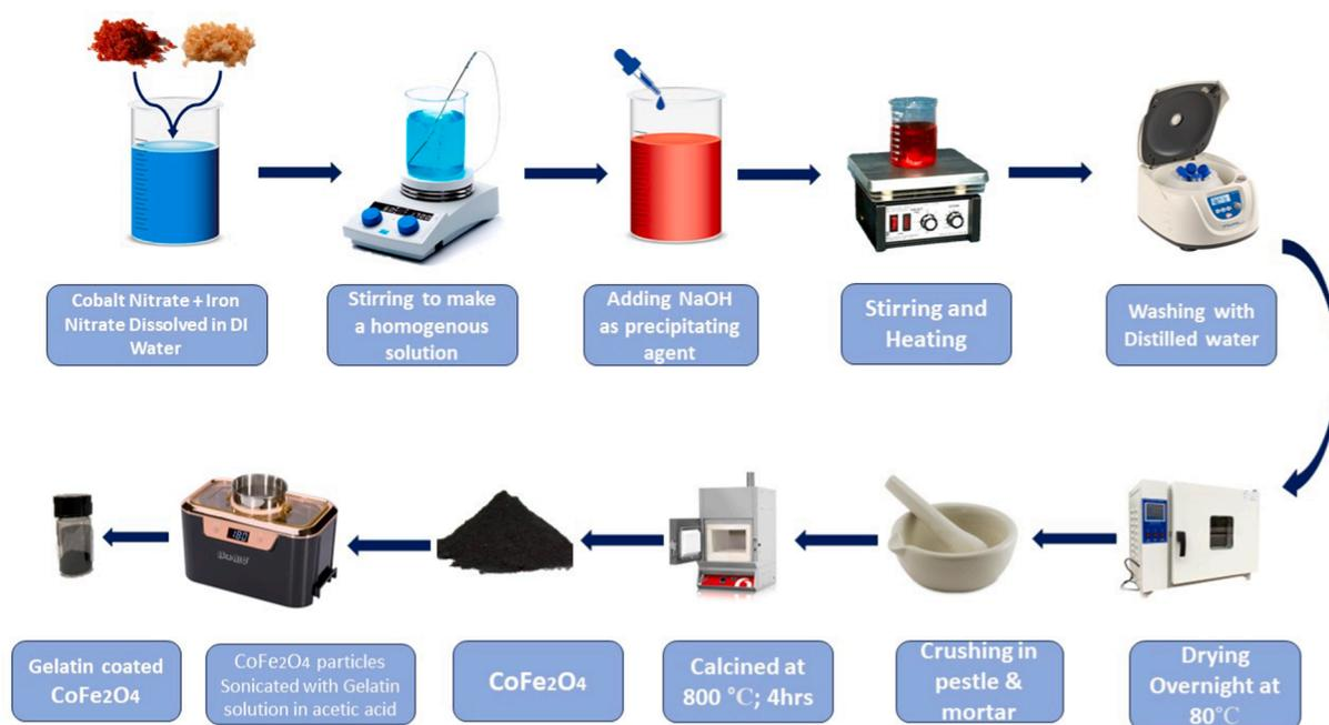
Fig. 1. Synthesis of spinel ferrites via co precipitation method.
