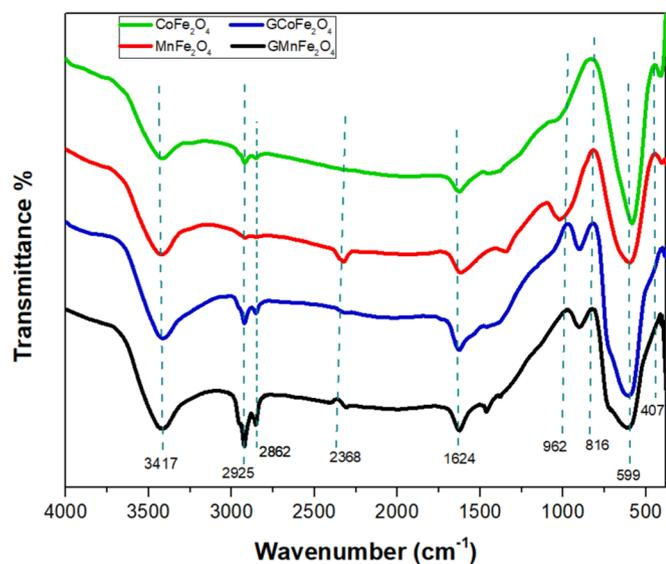
Fig. 5. The FTIR Spectra of Bare and Gelatin coated  $\text{CoFe}_2\text{O}_4$  and  $\text{MnFe}_2\text{O}_4$  Nanocomposites.
