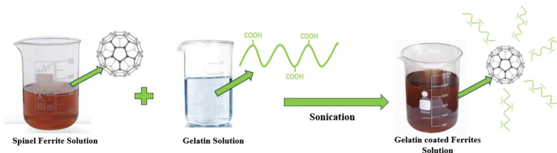
Fig. 2. Synthesis of gelatin coated spinel ferrites via Sonication.
