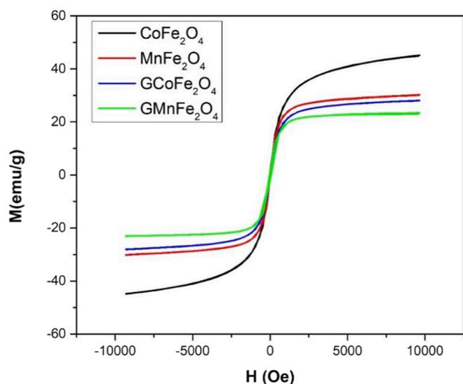
**Fig. 8.** Magnetic Hysteresis loop of Bare and Gelatin coated  $\text{CoFe}_2\text{O}_4$  and  $\text{MnFe}_2\text{O}_4$  Nanocomposites.
