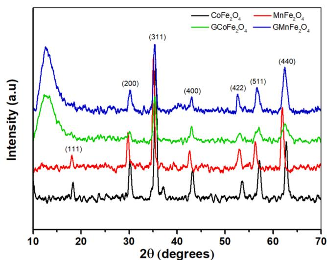
Fig. 3. The X-Ray diffraction Pattern of Bare and Gelatin coated CoFe<sub>2</sub>O<sub>4</sub> and MnFe<sub>2</sub>O<sub>4</sub> Nanocomposites.
