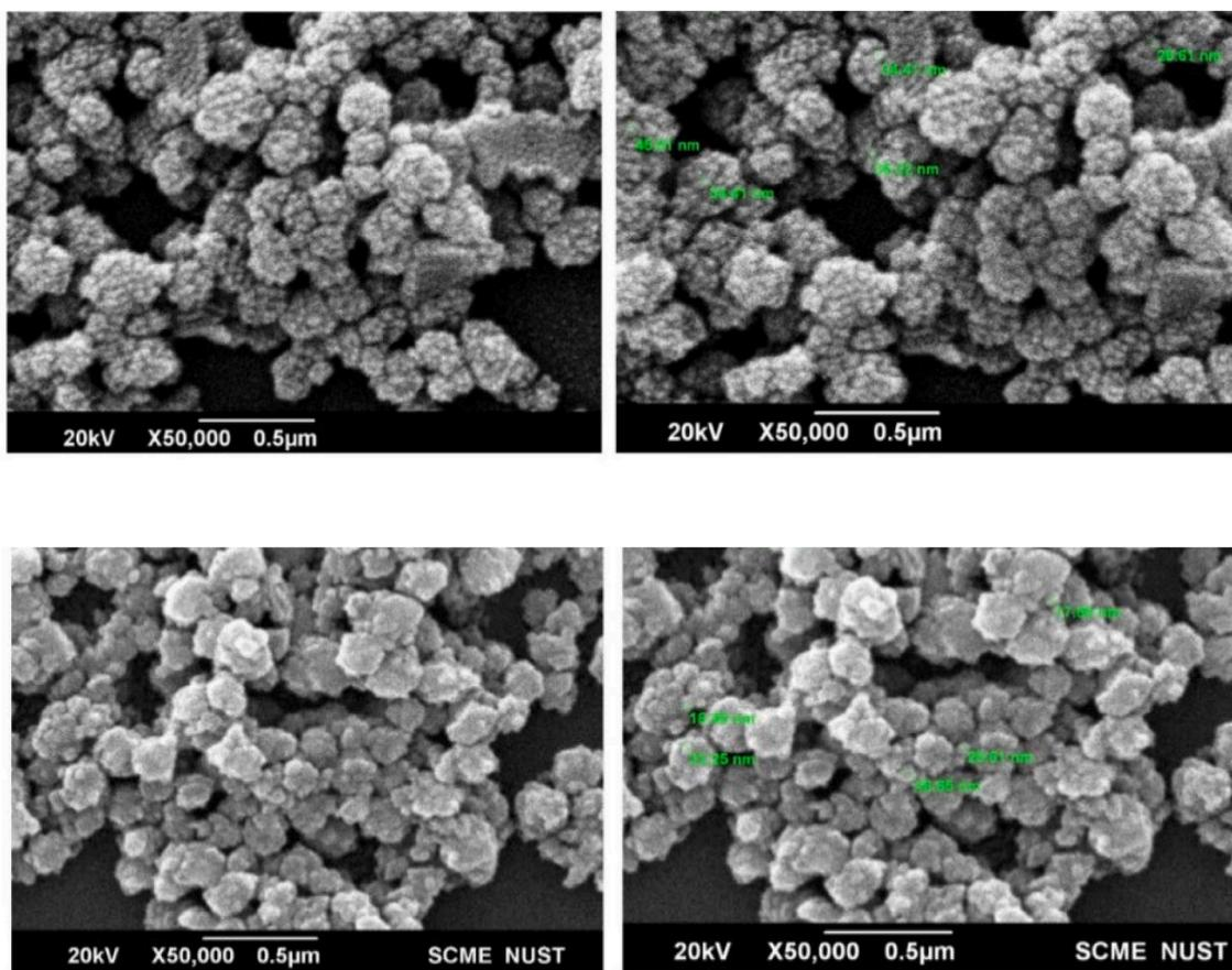
Fig. 4. SEM images of (a)  $\text{CoFe}_2\text{O}_4$  and (b)  $\text{MnFe}_2\text{O}_4$  Nanoparticles.
