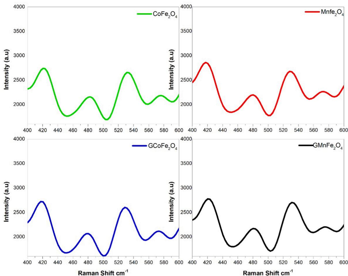
**Fig. 7.** The Raman Spectra of Bare and Gelatin coated  $\text{CoFe}_2\text{O}_4$  and  $\text{MnFe}_2\text{O}_4$  Nanocomposites.
