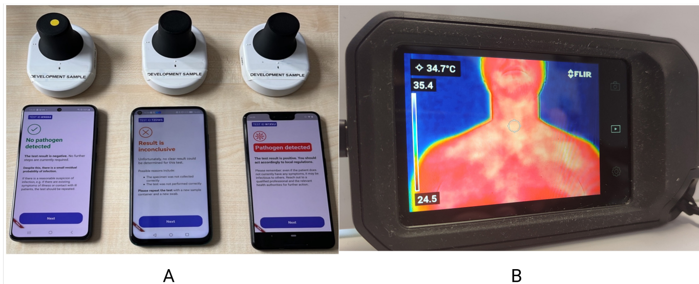
Figure 1 (A) Smartphones presenting three possible outcomes of the recombinase polymerase amplification assay in Minoo (Source: Dr Ahmed Abd El Wahed, doi: 10.1007/s15010-024-02179-z); (B) Thermal imaging device (camera) presenting with a thermography (Source: Dr Sophie Schneitler).
