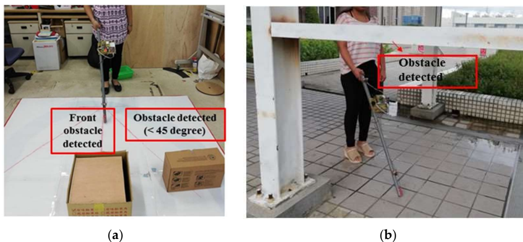
Figure 7. Experimental result of obstacle detection: (a) Indoor testing; (b) outdoor testing.
