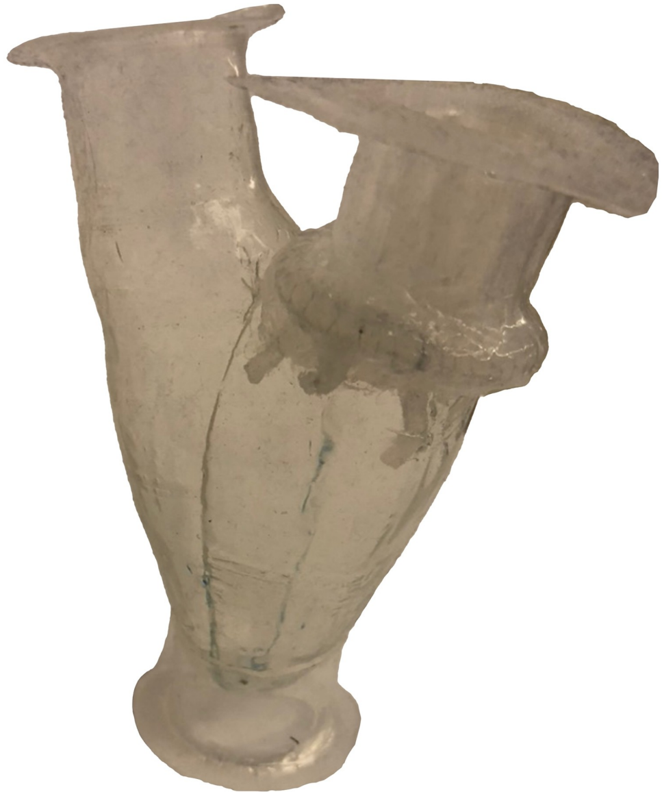
Fig 3. Left ventricular model. Completed left ventricular model with mitral valve sewn into the ventricle inlet, attached chordae, and silicone sealed layer.
