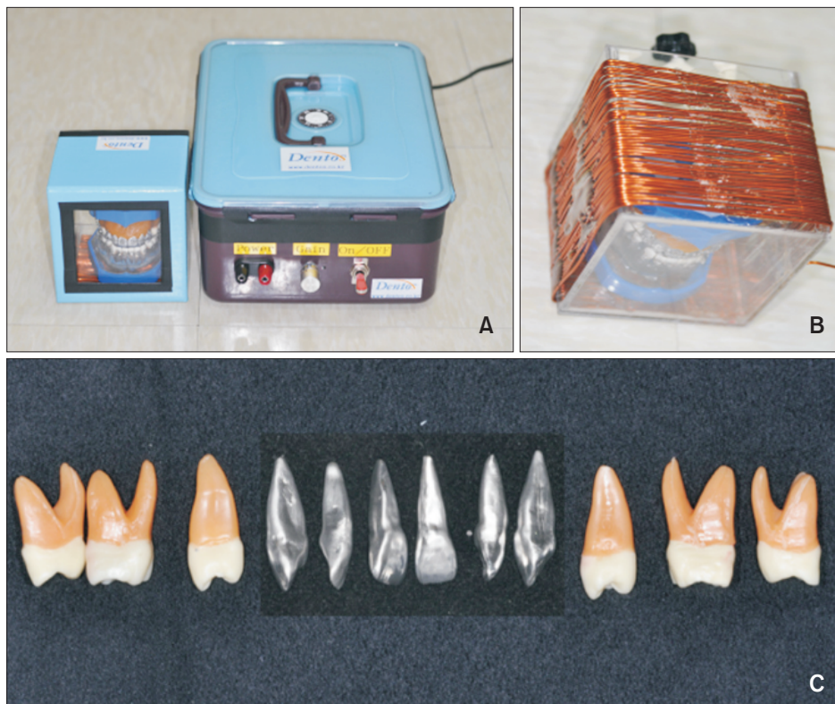
Figure 3. The new typodont simulation system. A, The overall set-up; B, the coil box; C, six aluminum anterior teeth and six resin posterior teeth.
