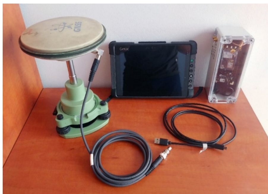
Figure 4. U-blox C099-F9P application board in self-made case with powerbank, Getac T800G2 rugged tablet with custom survey software, Leica AS10 antenna and cables.
