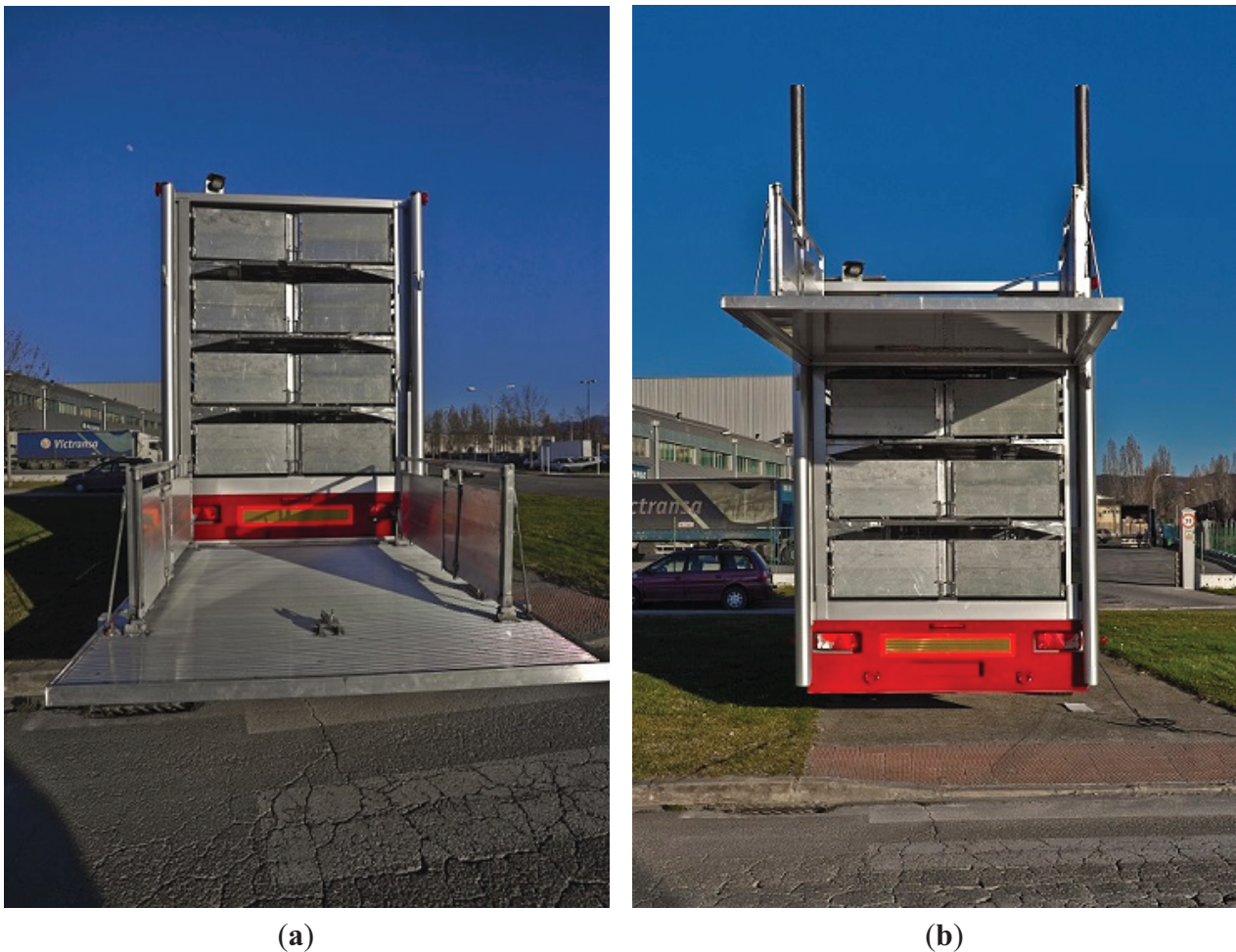
Figure 1. (a) Hydraulic lift elevator in the loading position. (b) Hydraulic lift elevator in the raised position.
