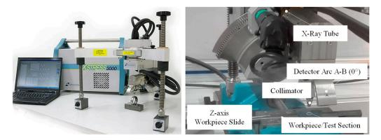
Figure 3. XRD analysis-basic system and measurement setup for wire workpiece.
