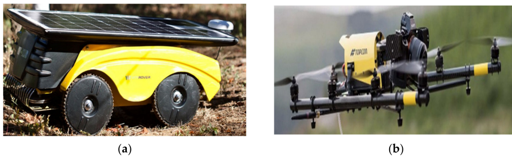
Figure 2. Image of solar-powered Vitirover robot in action on the ground (a); Falcon 8 drone employed to monitor, by means of the infrared (IR) sensors, the chlorophyll amount inside the vineyards (b).
