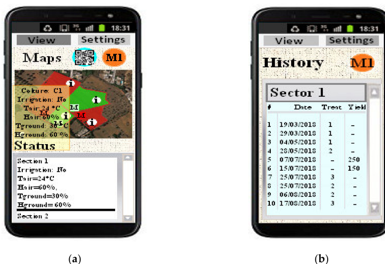
Figure 19. Screenshots of the realized application: “view section” where the farmer (user M1) has a complete overview of the cultivated crops (a) and “Data history section” through which the farmer or customer monitor crops’ parameters and the performed treatments for growth optimization (b).
