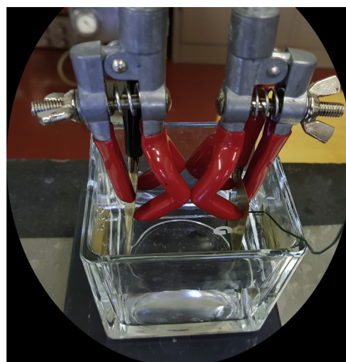
Figure 3 Specimen suspended with an insulated wire via a central hole in a glass containing 0.9% saline solution and in one-sided contact with one of two gold sheet electrodes (left and right).
