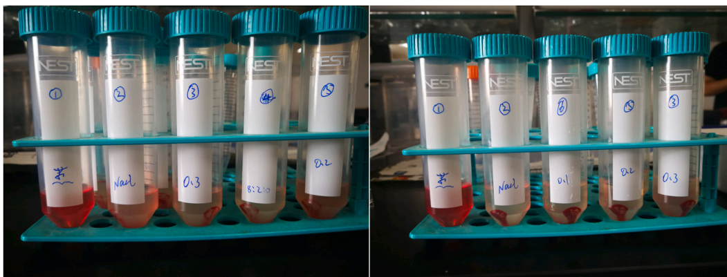
Fig. 12. Shows the hemolysis test results of four composite scaffolds. Note: tube 1 is the hemolysis test of distilled water in the positive control group. Hemolysis is positive and the liquid is light red; Tube 2 is the hemolysis test of normal saline in the negative control group, no obvious hemolysis is found, and the color of the solution has no obvious change. 3. Pipe 4, 5 and 6 are PCL respectively/ \beta - TCP/0.3%CNT, PCL/ \beta - TCP, PCL/ \beta - TCP/0.2%CNT, PCL/ \beta - In the hemolysis test of the extract of TCP/0.1% CNT composite scaffold, no obvious hemolysis was found, and the color of the solution did not change significantly. (For interpretation of the references to color in this figure legend, the reader is referred to the Web version of this article.)
