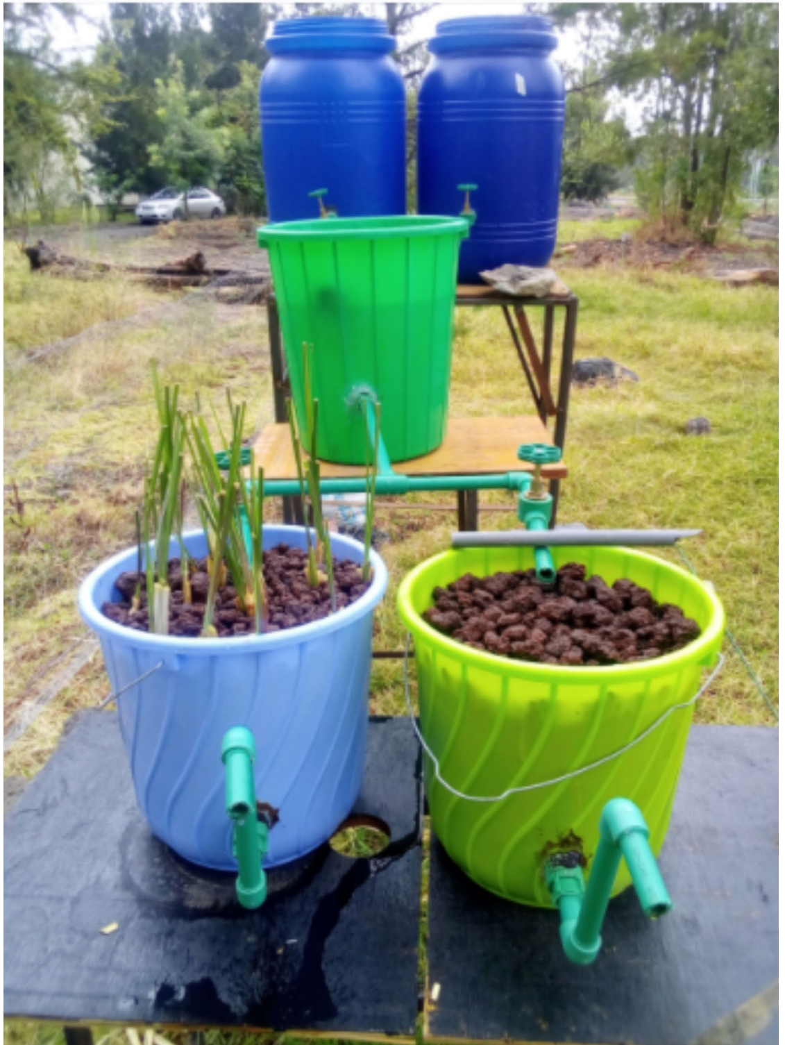
Fig. 2. The experimental setup of Vetiver grass planted VSSFCW and unplanted VSSFCW.
