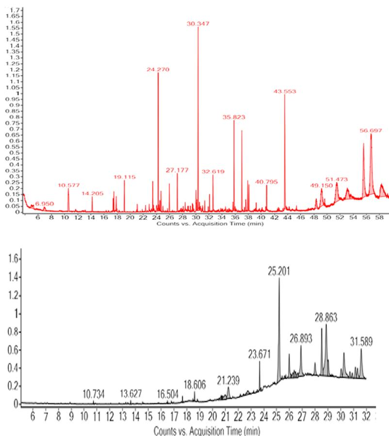
**Figure 1.** GC-MS chromatographic profile of ME (red) and EO (black) of *A. polystachyus*. The peaks indicate the major compounds, and the numbers above the peaks depict the retention time. The y-axis is for “intensity”.
