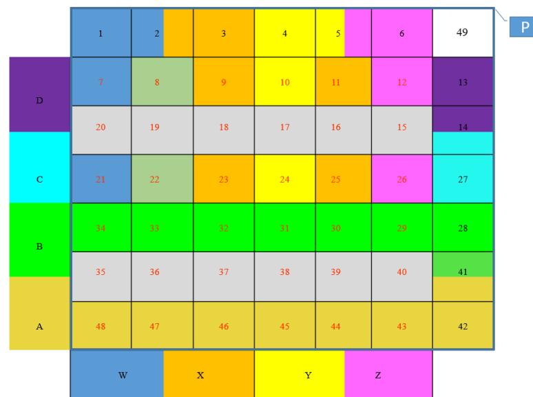
Figure 10. The 4 \times 4 sensors 2D array with overlapping arrangement of sensors A, B, C, D, W, X, Y, and Z, plus pressure sensor (P). Each color denotes the corresponding sensors in each tactel.
