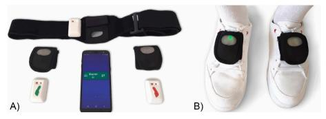
**Fig. 4.** Device components of the DeFOG system. A: Smartphone showing the step count and the three sensors with Velcro straps to attach them to the feet and chest. B: The feet sensors attached to the shoes.
