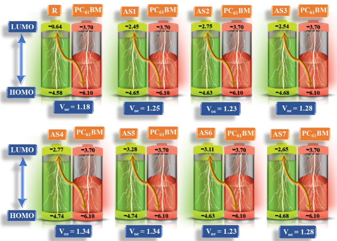
Figure 9. V_{oc} of the R and all modeled (AS1–AS7) molecules concerning the PC 61 BM acceptor polymer.
