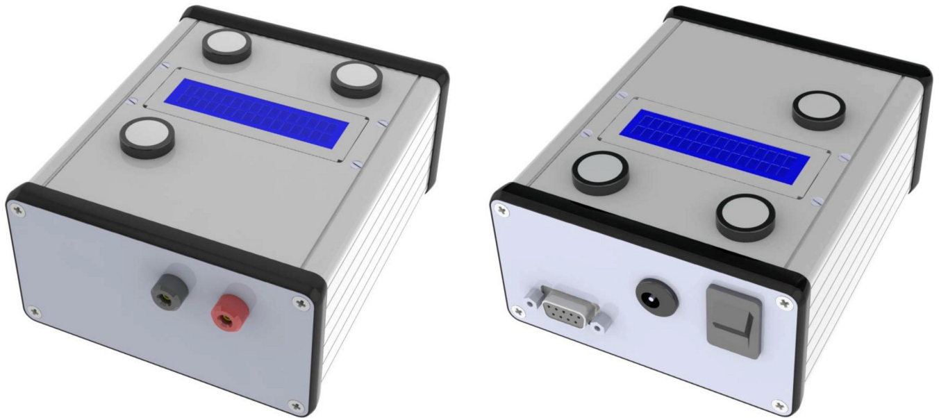
Fig 1. Open-tES stimulator overview. The front panel on the left side and the rear panel on the right side.
