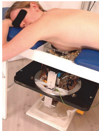
FIGURE 19: Clinical test with microwave radar-based system at Bristol University [25]. Image copyright IEEE, used with permission.
