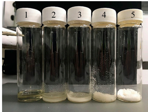
Figure 3. Photos of NMMO–IPA mixtures at room temperature with NMMO content: (1) 50; (2) 60; (3) 70; (4) 80; and (5) 90 (mass %).
