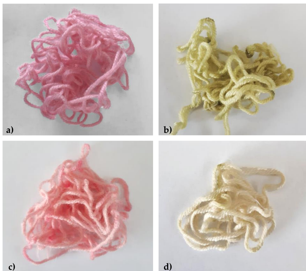
Figure 13. The visual appearance of dyed wool yarn samples before and after washing with a mildly alkaline reference detergent. (a) WoolP_1 before washing. (b) WoolG_1 after washing. (c) WoolP_2 before washing. (d) WoolG_2 after washing.
