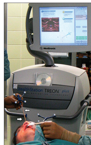
Figure 6: Navigation workstation. The navigation probe was calibrated for intraoperative computed tomography-tracking and direct visualization on the workstation's monitor by touching the operation field
