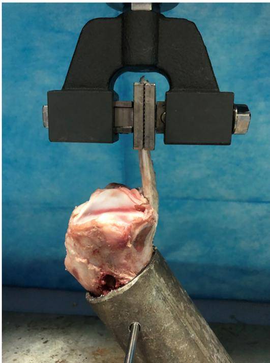
**Fig. 3** A specimen was fixed in an electronic universal biomechanical testing machine (AG-X; Shimadzu, Kyoto, Japan).
