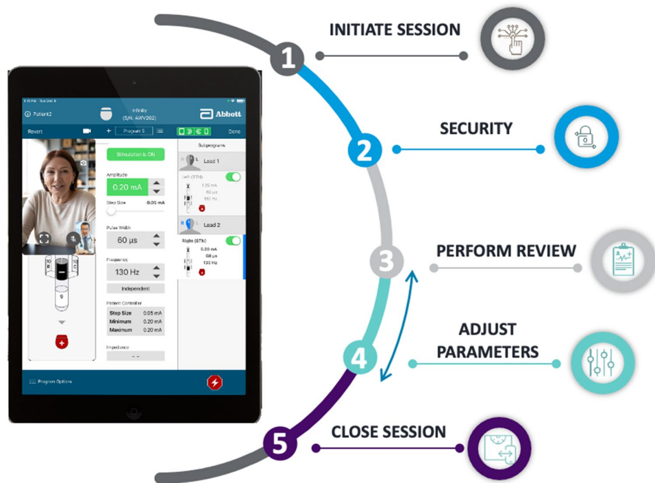
Figure 3. Clinical and communication workflow for a remote session. A typical remote care session using the remote care platform consists of the following steps: (1) session is initiated by the subject, (2) authentication of users and devices enabled via secure connection through the backend server, (3) review of symptoms and performance by the clinician, (4) iterative adjustment of programming parameters including amplitude, pulse width, frequency, and contact selection, (5) settings are saved, and session is closed by the clinician. *Individuals portrayed in the figure are not actual patients. Images are representative and taken from stock photos ( https://www.shutterstock.com/image-photo/head-shot-mature-woman-looking-camera-1720702294 ).
