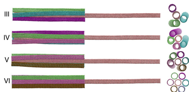
Figure 3. If a few atoms of outer CNTs are not fixed, rearrangement can be obtained in III, IV, and V cases. A sample snapshot of these systems has been presented. Just in VI case, there is no deviation.
