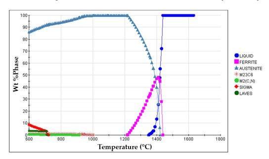
$\textbf{Figure 4.} \ \, \textbf{Equilibrium phase diagram of the GX5CrNiMo19-11-2 alloy (ISO 4991:2015) calculated with JMatPro^{TM} \ v.11.2 software. } \\$
