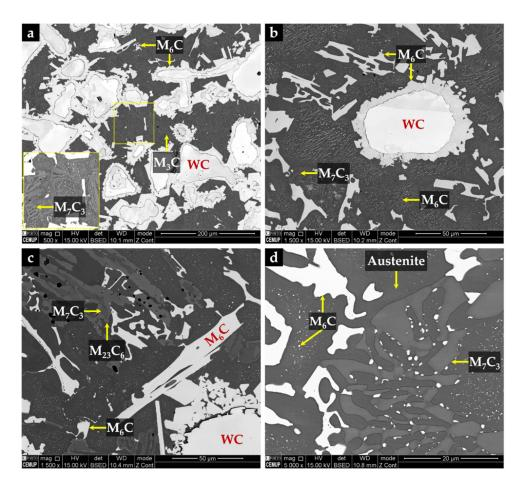
**Figure 18.** SEM-BSE images of the microstructure of CZ2 composite zone: (a)  $(Fe,W,Cr)_6C$  precipitated around WC particles, (b) higher magnification of (a) showing fine plate-like precipitation of  $(Fe,W,Cr)_6C$ , (c) carbides with a core of  $(Fe,Cr,W)_7C_3$  and a shell of  $(Fe,Cr,W)_{23}C_6$ , and (d) higher magnification of (c) showing the multi-phase interdendritic network.
