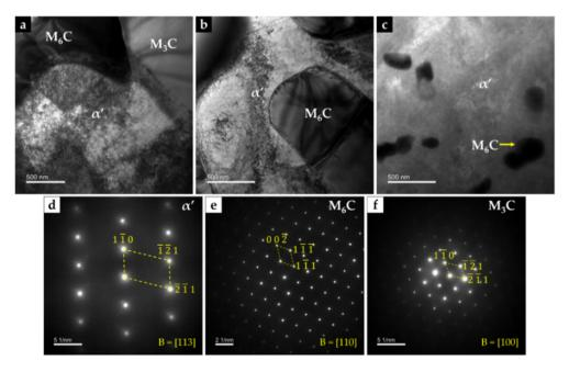
**Figure 17.** Dark-field TEM image of CZ1 composite zone: (a) interface between (Fe,W,Cr)<sub>6</sub>C, (Fe,W,Cr)<sub>3</sub>C, and  $\alpha'$ , (b) (Fe,W,Cr)<sub>6</sub>C with a quasi-cuboid shape precipitated within  $\alpha'$  matrix, and (c) fine precipitates of (Fe,W,Cr)<sub>6</sub>C. SAED patterns were achieved by using the (d) [113] zone axis for  $\alpha'$ , (e) [110] zone axis for (Fe,W,Cr)<sub>6</sub>C, and (f) [100] zone axis for (Fe,W,Cr)<sub>3</sub>C.
