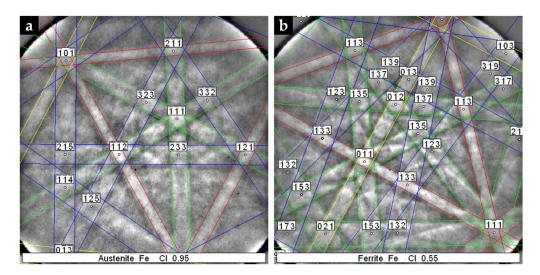
**Figure 11.** Indexed EBSD patterns corresponding to the phases that compose the microstructure of the austenitic stainless steel: austenite (**a**) and ferrite (**b**).
