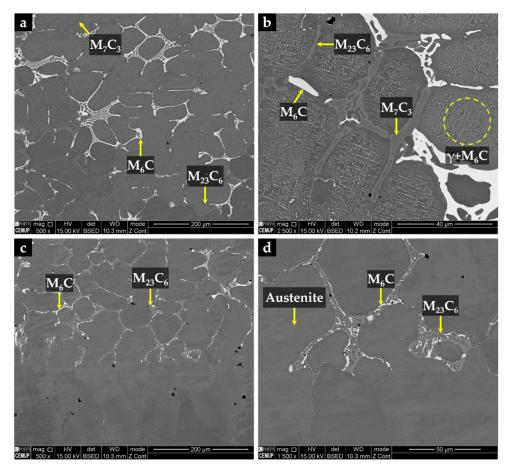
**Figure 20.** SEM-BSE images of the microstructure of CZ3 composite zone: (a) multi-phase interdendritic network of  $(Fe,Cr,W)_7C_3$ ,  $(Fe,Cr,W)_{23}C_6$ , and  $(Fe,W,Cr)_6C$ , (b) higher magnification of (a) showing fine precipitation of  $(Fe,W,Cr)_6C$  inside the  $\gamma$  matrix, (c) bonding interface free of discontinuities, and (d) higher magnification of (c) showing the interdendritic precipitation at the bonding interface.
