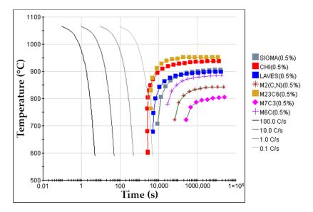
**Figure 5.** Continuous cooling transformation diagram (CCT) of GX5CrNiMo19-11-2 alloy (ISO 4991:2015) for an austenitizing temperature of 1075  $^{\circ}$ C, calculated with JMatPro<sup>TM</sup> v.11.2 software.
