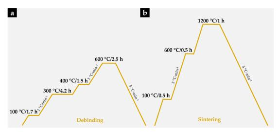
**Figure 2.** Debinding and sintering thermal cycles applied to Fe–WC compacts. (a) The thermal cycle carried out during debinding; (b) The applied thermal cycle with heating and cooling rates of  $5 \, ^{\circ}\text{C} \cdot \text{min}^{-1}$ .
