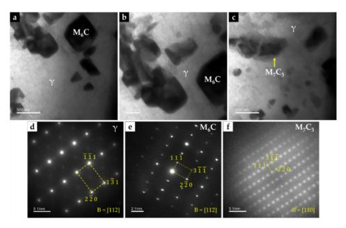
**Figure 21.** Bright-field TEM image of the CZ3 composite zone: (a)  $(Fe,W,Cr)_6C$  with a cuboid shape precipitated within  $\gamma$  matrix, (b) higher magnification of (a), showing an agglomerate of  $(Fe,W,Cr)_6C$  carbides, and (c)  $(Fe,Cr,W)_7C_3$  precipitated within  $\gamma$  matrix. SAED patterns were achieved by using the (d) [112] zone axis for  $\gamma$ , (e) [112] zone axis for  $(Fe,W,Cr)_6C$ , and (f) [110] zone axis for  $(Fe,Cr,W)_7C_3$ .
