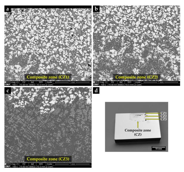
**Figure 13.** SEM-BSE images of the microstructure of the reinforced specimen showing three zones: composite zone nearest to the surface—CZ1 (a), intermediate composite zone—CZ2 (b), composite zone next to the base metal—CZ3 (c), and a cross-section of the specimen with the identified zones (d).
