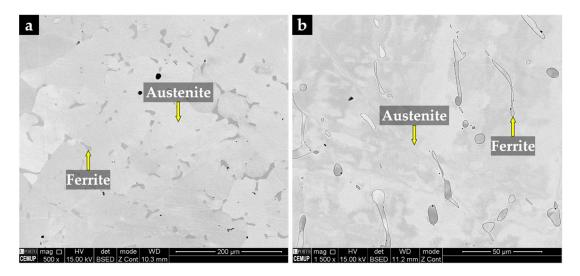
**Figure 10.** SEM image of the austenitic stainless steel after solution heat treatment at 1075  $^{\circ}$ C/2 h (a) and the same after chemical etching with 10% oxalic acid and higher magnification (b).
