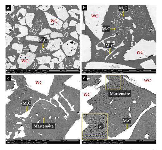
**Figure 16.** SEM-BSE images of the microstructure of the CZ1 composite zone: (a) uniform distribution of large polygonal-shaped WC particles and small particles of  $(Fe,W,Cr)_6C$ , (b) higher magnification of (a) showing fine precipitation of  $(Fe,W,Cr)_3C$  and  $(Fe,W,Cr)_6C$ , (c)  $\alpha'$  matrix revealed with 10% oxalic acid, and (d) higher magnification of (c) showing the  $\alpha'$  plate-like morphology.
