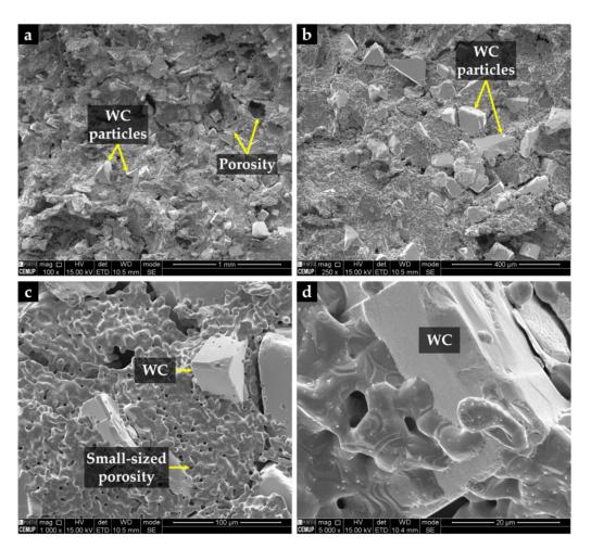
**Figure 7.** SEM-SE images of the surface of the porous sintered Fe–WC inserts: (a) Fe matrix with large WC particles and random porosity, (b) large polygonal-shaped WC particles with higher magnification, (c) small-sized porosity, and (d) wetting of a large WC particle by the iron.
