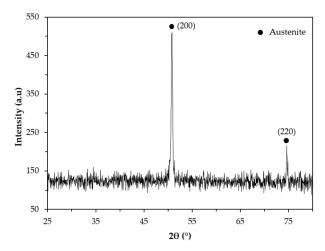
**Figure 9.** X-ray diffraction (XRD) pattern of the base metal in the  $2\theta$  range of  $25^{\circ}$ – $80^{\circ}$ .
