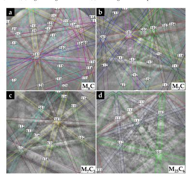
**Figure 19.** Indexed EBSD patterns of the carbides in CZ2 composite zone:  $(Fe,W,Cr)_6C$  (a),  $(Fe,W,Cr)_3C$  (b),  $(Fe,Cr,W)_7C_3$  (c), and  $(Fe,Cr,W)_{23}C_6$  (d).
