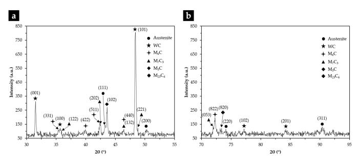
**Figure 15.** XRD patterns of the composite zone in the  $2\theta$  range of  $30–55^{\circ}$  (a), and  $70–95^{\circ}$  (b).
