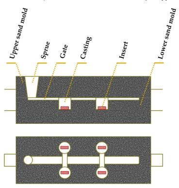
Figure 3. Scheme of the mold with the Fe–WC inserts (side and top views) (adapted from [40]).
