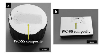
**Figure 8.** The reinforced specimen (a) and a cut through the cross-section (b), showing the depth of the composite zone.
