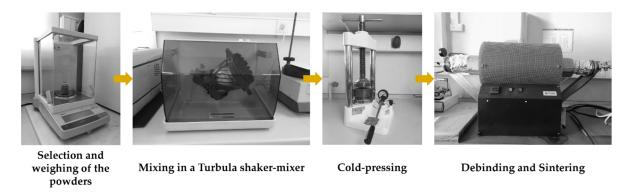
Figure 1. Fabrication steps for the Fe–WC inserts production.
