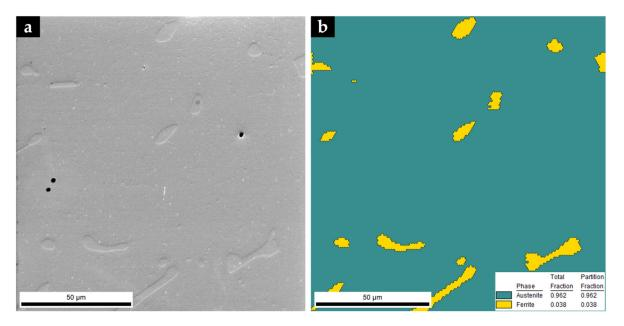
**Figure 12.** SEM image of the microstructure of the base metal (a) and EBSD phase map:  $\gamma$  in dark cyan and  $\alpha$  in yellow (b).
