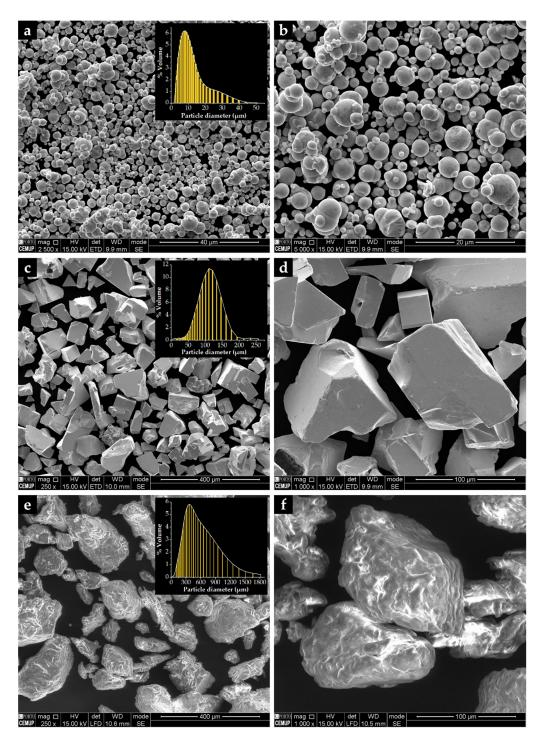
**Figure 6.** SEM-secondary electron (SE) images of the starting powders: (**a**,**b**) Fe with round morphology, (**c**,**d**) polyhedral particles of WC, and (**e**,**f**) M0101 binder with irregular shapes.
