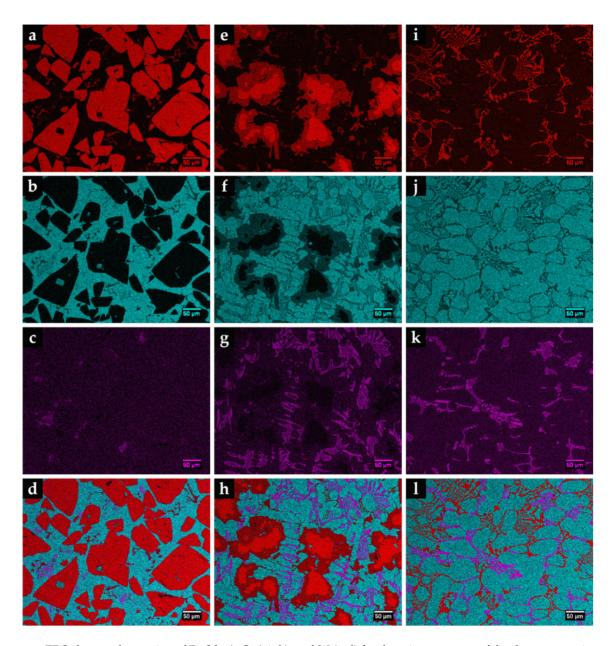
**Figure 14.** EDS elemental mapping of Fe (blue), Cr (pink), and W (red) for the microstructure of the three composite zones: CZ1 (a–d), CZ2 (e–h), and CZ3 (i–l).
