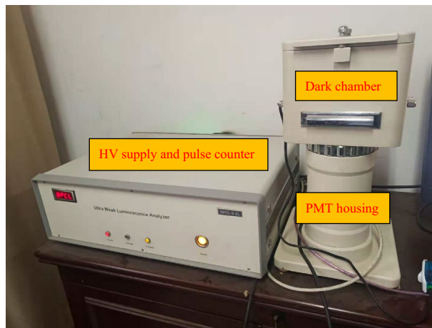
Figure 2. Ultra weak luminescence measurement instrument used in the experiment.
