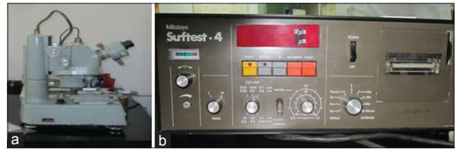
Figure 5: (a) Vickers Microhardness tester: Shimadzu, Japan, (b) Profilometer: Mitutoyo surfest-4
